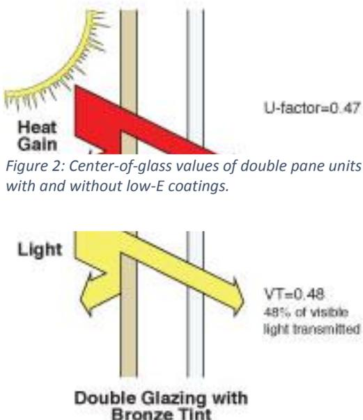
Figure 2: Center-of-glass values of double pane units with and without low-E coatings.
