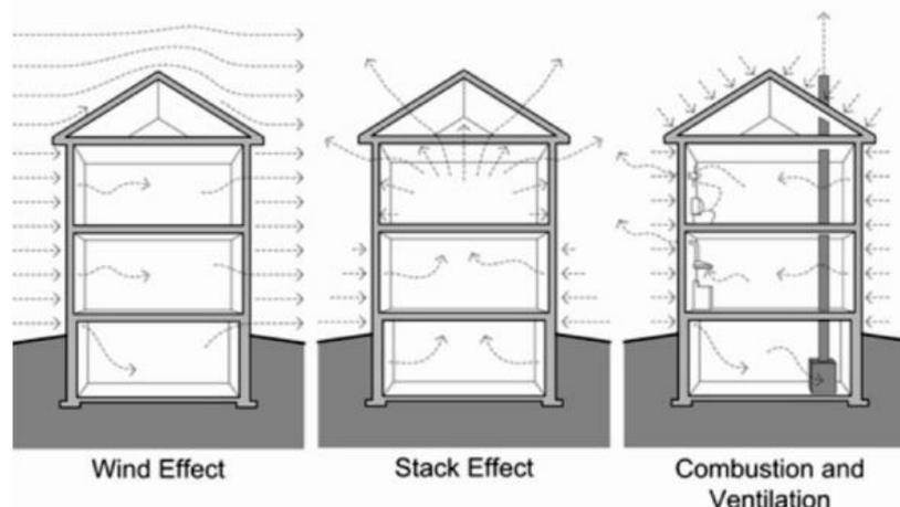
Figure 1: Examples of infiltration. Image courtesy: Building Science Corporation, [www.buildingscience.com](http://www.buildingscience.com)
