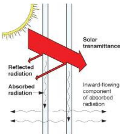
Figure 1: Simplified view of the components of solar heat gain. Heat gain includes the transmitted solar energy and the inward flowing component of absorbed radiation.
